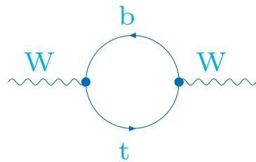
$$\Delta\rho_{\text{top}} \sim \frac{\Sigma_T^{ZZ}(0)}{M_Z^2} - \frac{\Sigma_T^{WW}(0)}{M_W^2} \sim \frac{3G_\mu m_t^2}{8\sqrt{2}\pi^2}$$
