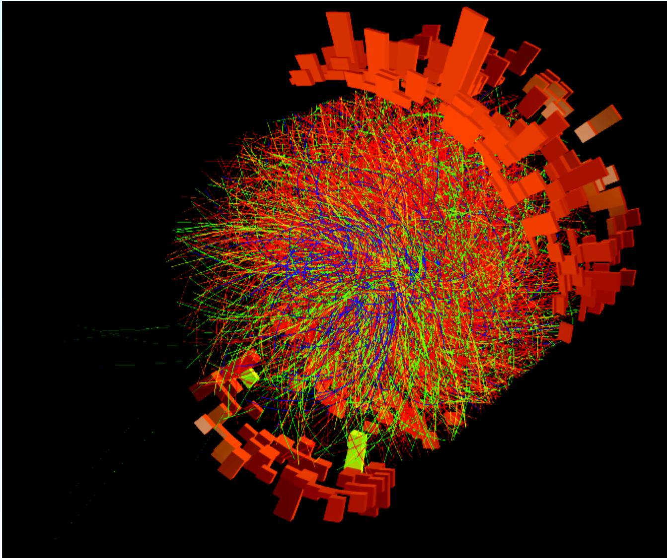
Tracks of particles recorded with the Time Projection Chamber and clusters in the calorimeter for a Pb-Pb collision at  $\sqrt{s_{NN}} = 5.02$  TeV
