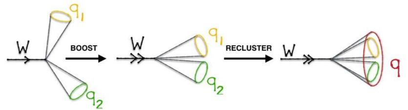
Within the 0-Lepton SUSY analysis, a set of dedicated signal regions has been developed and optimised, exploiting the selection on the large-R jets obtained from a particular algorithm called **Reclustering**, which is able to form a large jet from the usual small ones taken as inputs.
