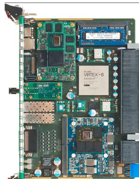
TIGER – A programmable digital trigger and readout concentrator VXS-switch board
